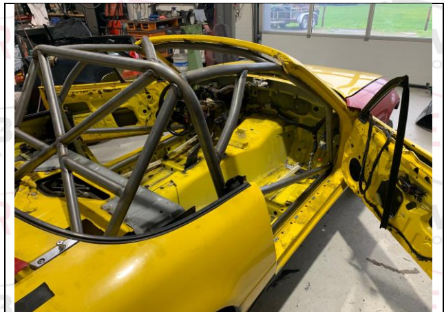
PHOTO 12 ANTI-INTRUSION DOORBAR – CO-DRIVER
