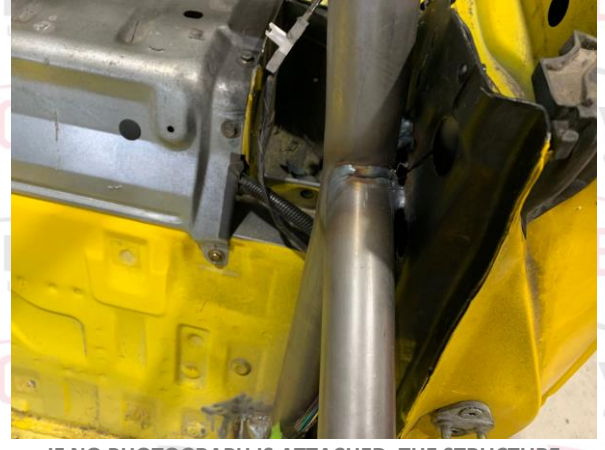
PHOTO 8 MAIN ROLLBAR TO "B" PILLAR ATTACHMENT
