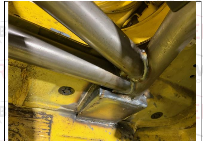
PHOTO 6 FRONT ROLLBAR TO FLOOR ATTACHMENT
