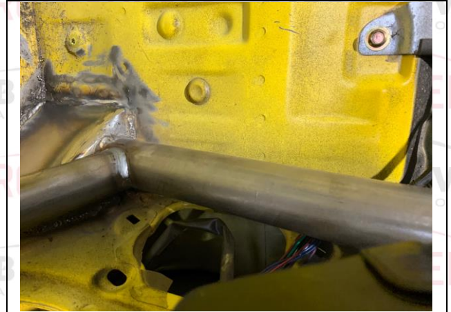
PHOTO 4 MAIN ROLLBAR TO FLOOR ATTACHMENT
