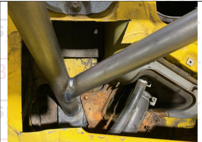
PHOTO 5 REAR BACKSTAY TO BODYSHELL ATTACHMENT
